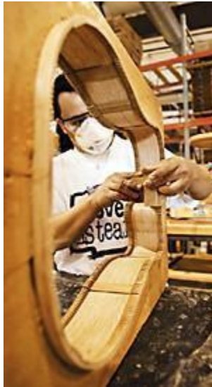
Yunpok Yi examines the neck of an instrument before he goes back to sanding and adjusting it to make sure it's in perfect alignment with the bridge of the guitar.
