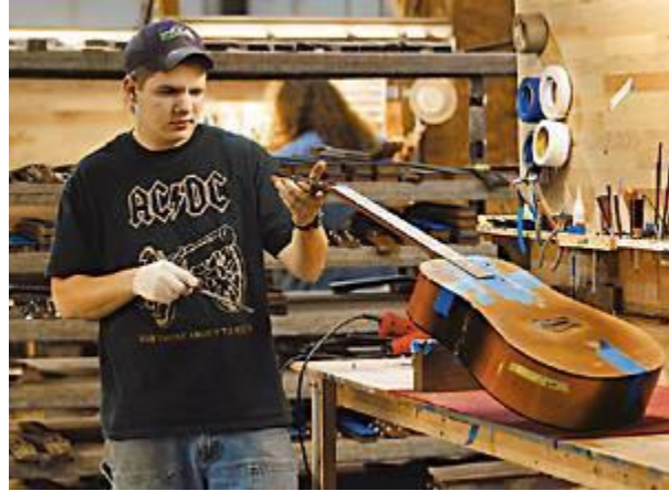
Simon Nielson files down the raised frets until each one is aligned perfectly with the rest. A wood cover is put over the top of the guitar so it isn't damaged during the filing.
