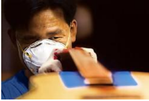
Yunpok Yi examines the neck of an instrument before he goes back to sanding and adjusting it to make sure it's in perfect alignment with the bridge of the guitar.
